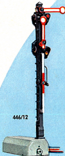
446/13 Home Signal with two independent arms · Operation, connections and track current control as with all signals for train control, but with an additional third solenoid · The current returns through an extra blue lead with an orange cross plug-in connection. Through the mechanical interconnection of the two armatures the three possible signal indications are provided by supplying current to one solenoid only in each case · Light change either from red to green or red to green/orange · Width 1 in., length 4¾ in., height 5 in.
