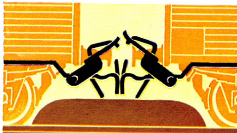
Raising the ramps releases the coupling.
