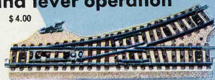
Manually-worked pair of points · Finished with rail crossings, guide rails and so on · Spring tongues for the points · Track sizes the same as 5117
