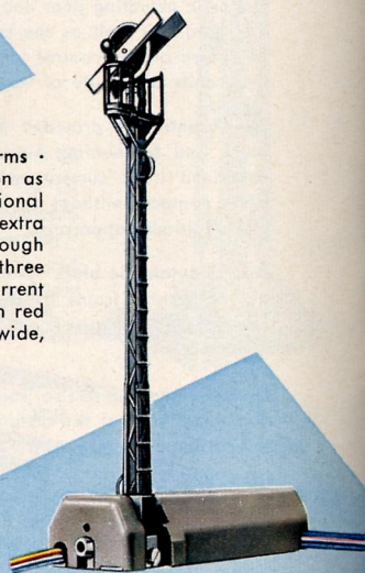
7043 $ 7.25 Fly-shunting Signal. The signal arm shows three indications, "Stop", "Shunt slowly" and "Shunt moderately fast". In the "Stop" position the track current is cut off, but is switched on in the other two positions. The cable connections are yellow with yellow plugs, blue with red plugs, blue with green plugs and blue with orange plugs. 1 1/8 in. wide, 3 3/8 in. long, 5 1/8 in. high
