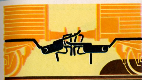
The couplings are uncoupled by raising an actuating ramp between the rails
