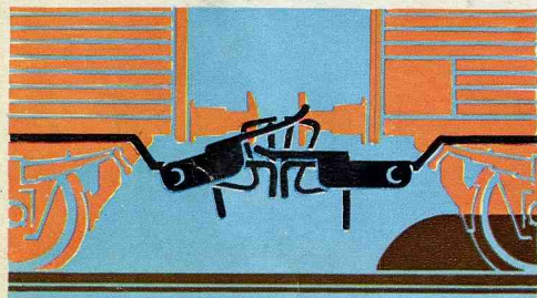
Raising the ramps releases the coupling.
