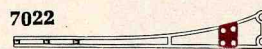
7022 ▲ Interrupter cam section for interrupting the overhead contact wire current (for push-in connection) · 4 1/2 in. long
