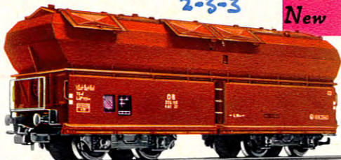
High-capacity Goods Truck with hinged cover roof, a model of the German Federal Railways' eight-wheeled KKt 57 type truck · Finished brown; all covers to open · 5 1/2 in. long
