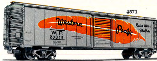
Box Car , a model of the Western Pacific Railroad's 50-ton eight-wheeled car · The model has bogies with movable bolsters and a detachable roof with fixed walkway, doors both sides to open · Finished silver grey · 8 1 / 8 in. long
