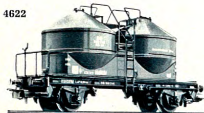
Container Truck for Fine Bulk Goods , a model of the German Federal Railways' four-wheeled Kds 54 type · The model has grey containers, shaded white with a black underframe · Approximately 4 in. long
