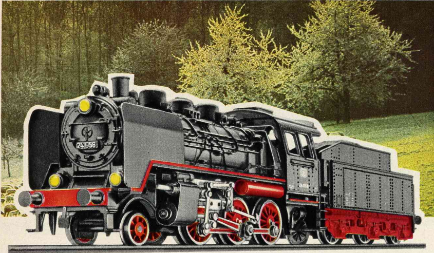
The standard Class 24 locomotive was used on the German Federal Railways for passenger and goods services, its maximum speed being 56 miles an hour.
