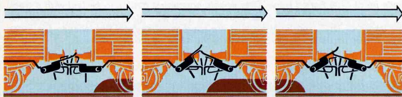
Raising the track ramp releases the couplers.
