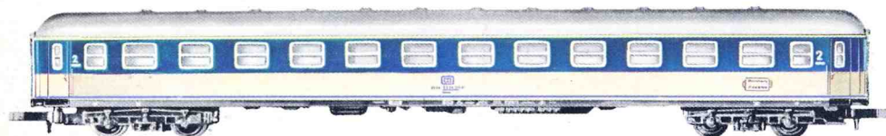
8721 Express car · 2nd class · A model of a German Federal Railways' car (B üm) · Windows inset in plastic frames · 4 7 / 8 " long
