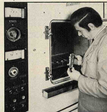
Materials testing under extreme climatic conditions in a temperature and humidity-controlled cabinet.
