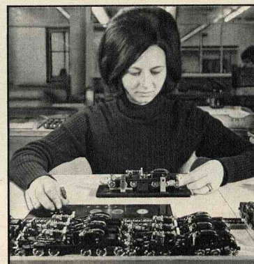
Adjustment of the reversing switch and testing the operation of the locomotive.
