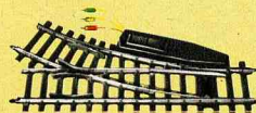
Solenoid-operated right-hand turnout · Operated by double solenoid · Sprung switch points · Turnout angle 30° · Radius of branch track 600 mm · Length of straight track section 300 mm
