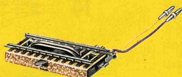
5112 Uncoupling track section for releasing automatic couplings · When the button on the control box is pressed, the solenoid-operated ramps on either side of the stud contacts are raised, releasing the couplings · 2 connecting leads · Length of track 90 mm
