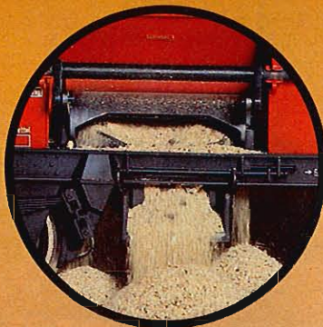
Operating rotary bar trips hoppers
