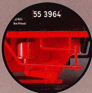
Free standing piping at the cab
