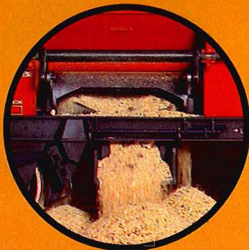
Operating rotary bar trips hoppers
