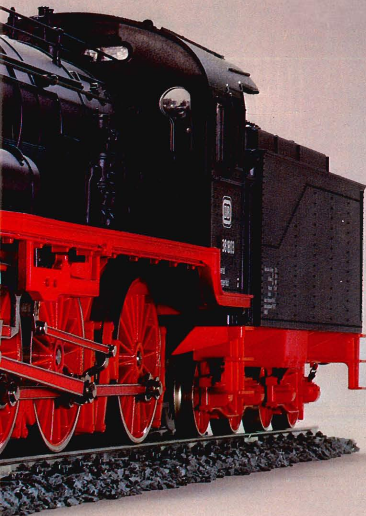
Sprung buffers, prototypical screw couplers, and simulated air brake hoses
