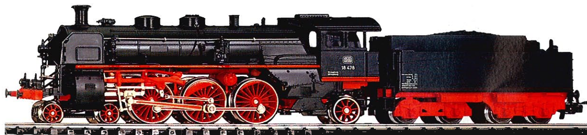
3093 · Express Locomotive with Tender · German Federal Railroad class 18 4 (ex-S 3/6) · 3 axes powered by means of connecting rods · 2 traction tires · Illuminated triple headlight · Metal body and frame · RELEX coupler on tender · Length over buffers 24.9 cm (9-13/16") · Equipped for installation of smoke unit (Seuthe No. 20) Ⓞ = 7152 🚂 = 7185 ♁ = 60015
