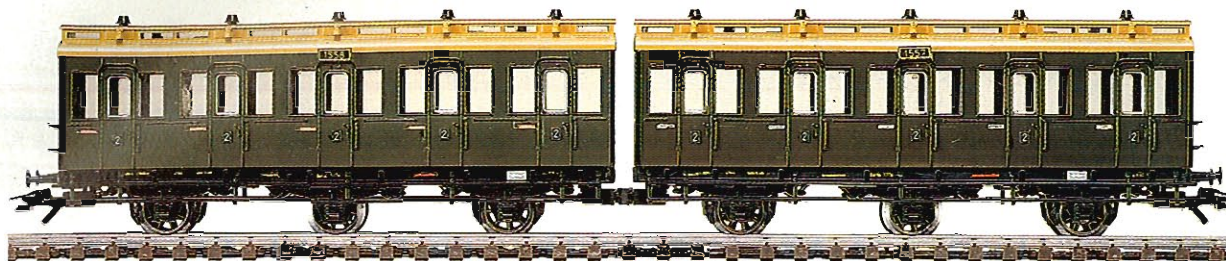
4207 · Double Compartment Car · B3/B3 for the Berlin Metropolitan Railroad · 2 nd class · Interior details · Permanent close coupling between the two car halves · Automatic close couplers at the car ends · Length 26.4 cm (10-3/8")
