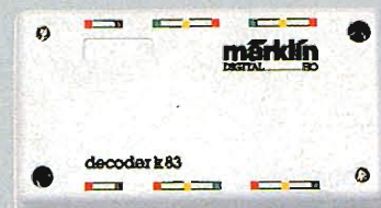
6083 Decoder k 83 4" x 2" x 1" / 100 x 54 x 22 mm
