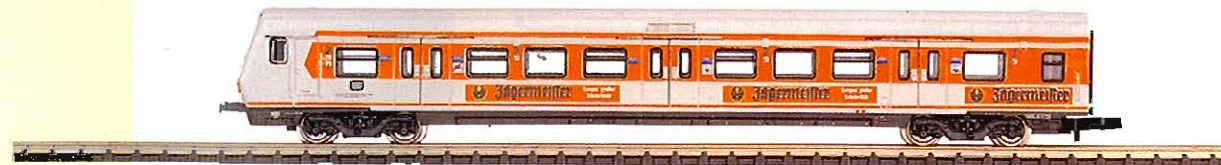
N 87990 S-Bahn Car with Control Cab. Bxf 796.1 with advertising along the car's sides for "Jägermeister". 2nd class. Length over buffers 115 mm (4-1/2").
