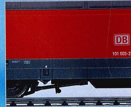
Movable mechanical gear for steering the trucks.
