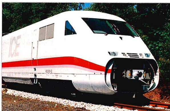
Automatic couplers enable quick uncoupling and coupling of the ICE 2 train halves.
