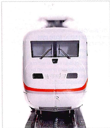
Front view of the ICE 2 powered end unit with closed nose plates.
