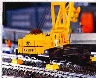
Counterweights mounted on the crane superstructure.
