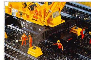
Support arms swung out into position – crane in working position.
