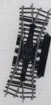
2260 Double Slip Switch. With detachable solenoid mechanism (7549). Crossing angle 22° 30'. Curve same as 2232. Length of straight side 168,9 mm / 6-5/8".
