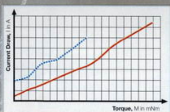
Compared to the traditional motor, the C-Sine motor has a clearly lower current draw.
