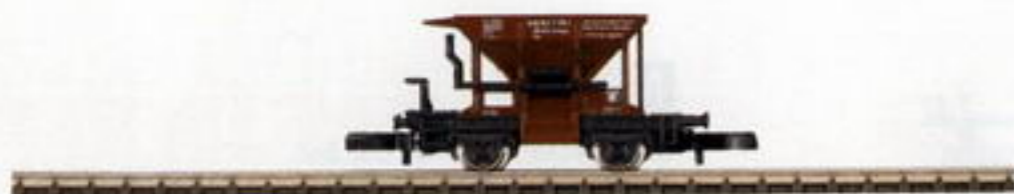
IV 8624 Ballast Car. Prototype: Talbot self-dumping car for maintenance work on the German Federal Railroad (DB). Model: Unloading hatches that can be opened. Length over buffers 33 mm / 1-5/16".
