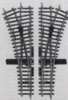
2265 (2264 L) Left Turnout. 2266 (2264 R) Right Turnout. With detachable hand levers. Turnout branch 22° 30'. Branch same as 2232. Length of straight side 168,9 mm / 6-5/8". 7549 solenoid mechanism can be installed on these turnouts.
