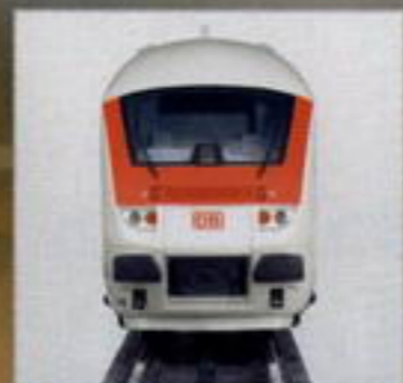
When operated locomotive first, dual red marker lights shine.
