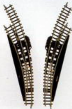
8568 L Electric Left Curved Turnout. 8569 R Electric Right Curved Turnout. Radius 195 mm / 7-11/16". 30° (same as 8521.) Main track length 25 mm / 1".
