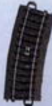
24194 Curved Circuit Track R1 = 360 mm / 14-3/16" / 15°. Momentary contact by means of locomotive/ car pickup shoe.
