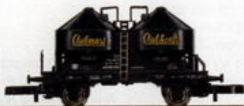
III 86661 Silo Container Car. Prototype: Type Ucs 909. Car privately owned by Club-Kraftfutterwerke GmbH, Mannheim, Germany. Used on the German Federal Railroad (DB). Model: Length over buffers 40 mm / 1-9/16".
