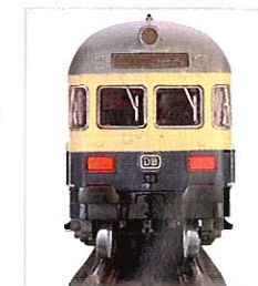
When operated cab control car last, dual red marker lights shine.
