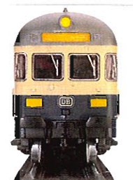
When operated cab control car first, triple white headlights shine.
