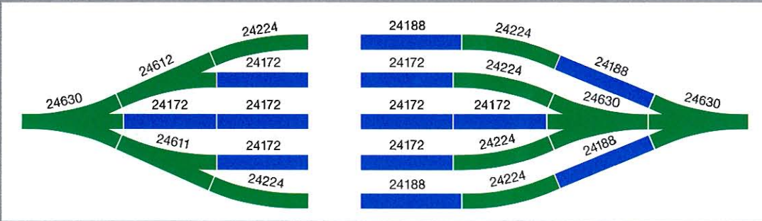
Offset arrangement of the switch rails
