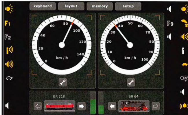
Representation of locomotives with color images, up to 16 controllable functions, graphic representation of the settings for these functions.
