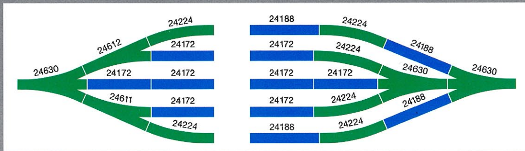
Offset arrangement of the switch rails
