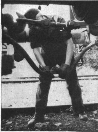
Connecting the Air Brake Pipe when coupling coaches
