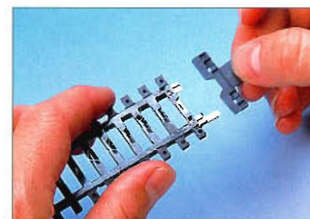
8 & 9. Insulating the third rail on K Track.
