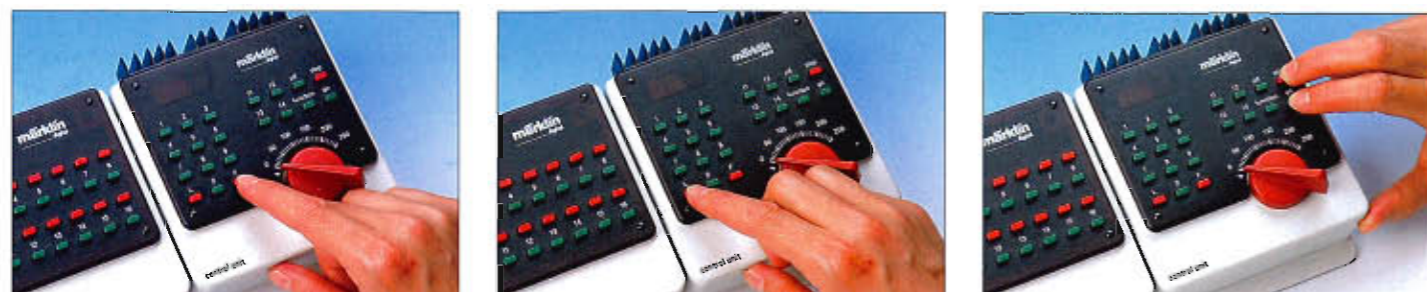
1, 2 & 3. From left to right: Pressing the button F = selecting a Function; pressing the button L = selecting a Locomotive; pressing Reset with "stop" and "go"
