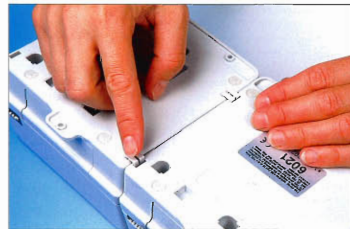
1, 2 & 3. The Keyboard is plugged in on the left side of the central unit and is fixed in place with clips on the bottom of the units.
