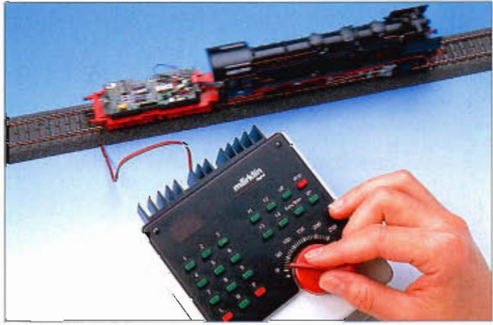
4. Changing the address set at the factory to one of your own choice; and braking delays as well as the speed control on ascending and descending grades;
