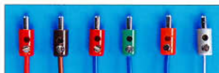
12. Below: Plugs and wires in the appropriate combinations.
