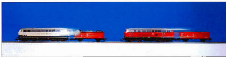
8. Above: The acceleration for specific trains can be set with the c 90 decoder. A loaded freight train (left) travels more slowly than an unloaded one (right). In addition, the maximum speed can be held nearly constant.
