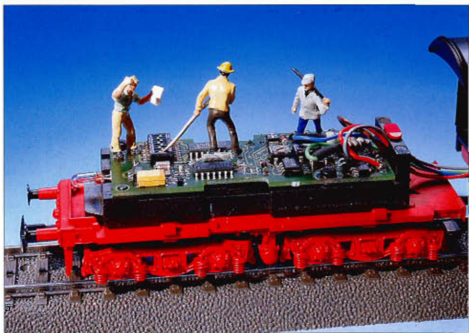
2. Below: Setting the digital address with the eight coding switches
