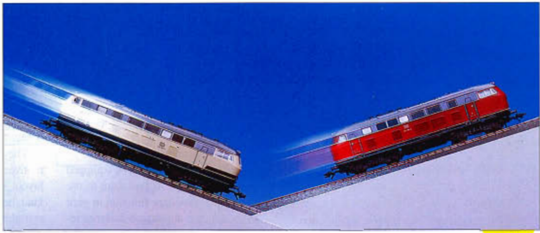
8. Above: The acceleration for specific trains can be set with the c 90 decoder. A loaded freight train (left) travels more slowly than an unloaded one (right). In addition, the maximum speed can be held nearly constant.
