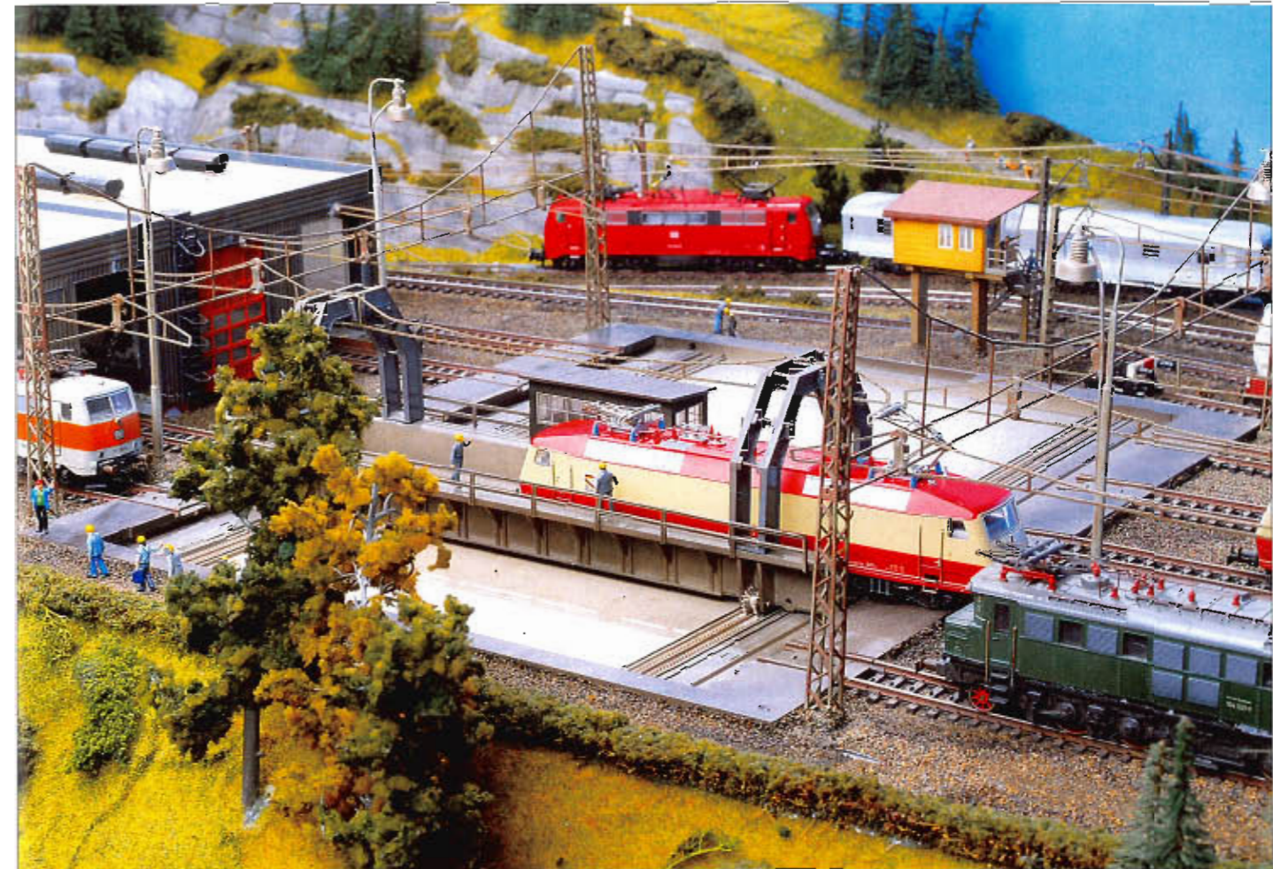
9. With the special catenary set the transfer table can also be used for electric locomotives. It requires less space than a turntable. With digital control there are all sorts of applications for the transfer table.
