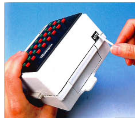
4. Connecting a k 84 decoder to the Control Unit
