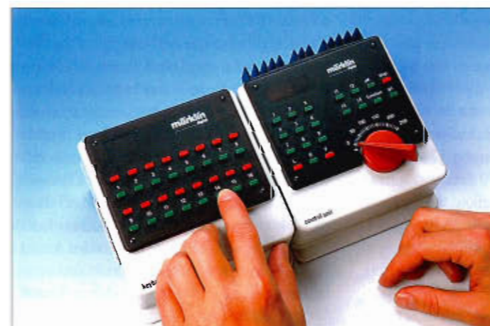
6 & 7. Pressing the green button sets the signal for "go", pressing the red one sets its for "stop".
