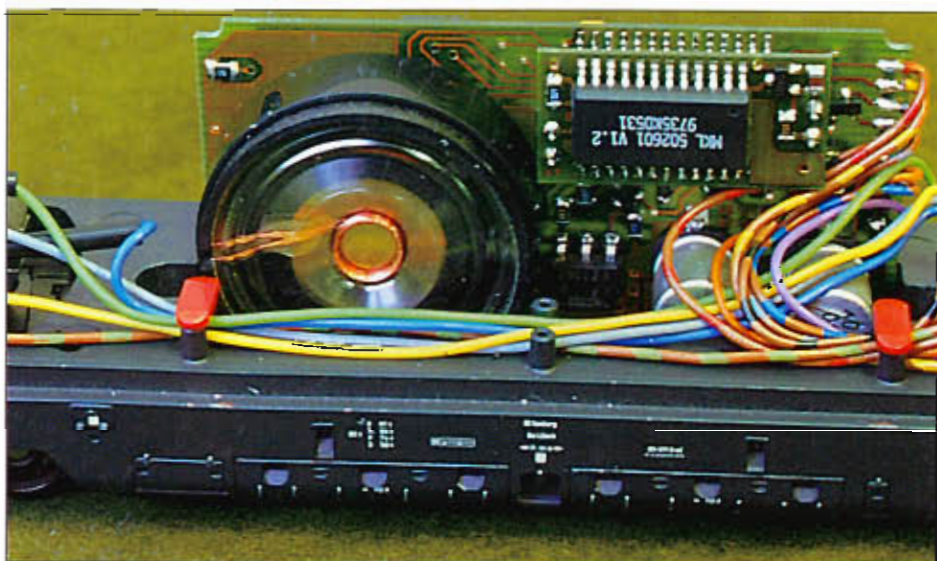
Above & Right On locomotive 37803, the volume of the signal horn is regulated using the left potentiometer while the right one regulates the volume of the diesel engine. The sound module can be individually regulated via this coding switch.
