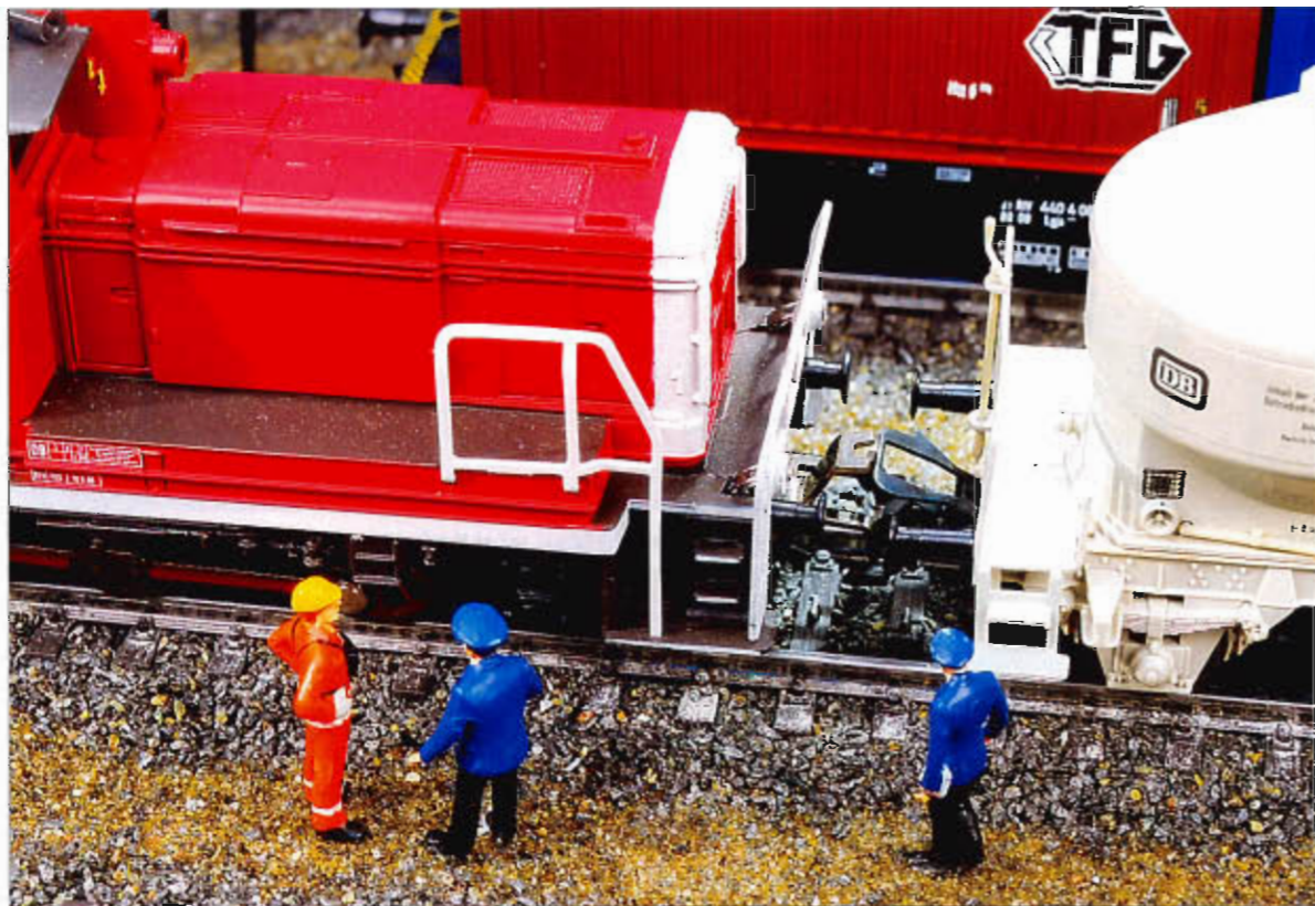
10. Irritation in the switch yard. The switchman, accused of sleeping on the job, explains to his superior, why he is no longer required for uncoupling: the class V 60 switch engine has TELEX couplers!
