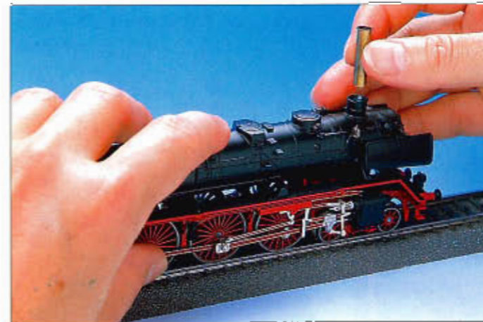
12. Installing the Seuthe smoke generator
